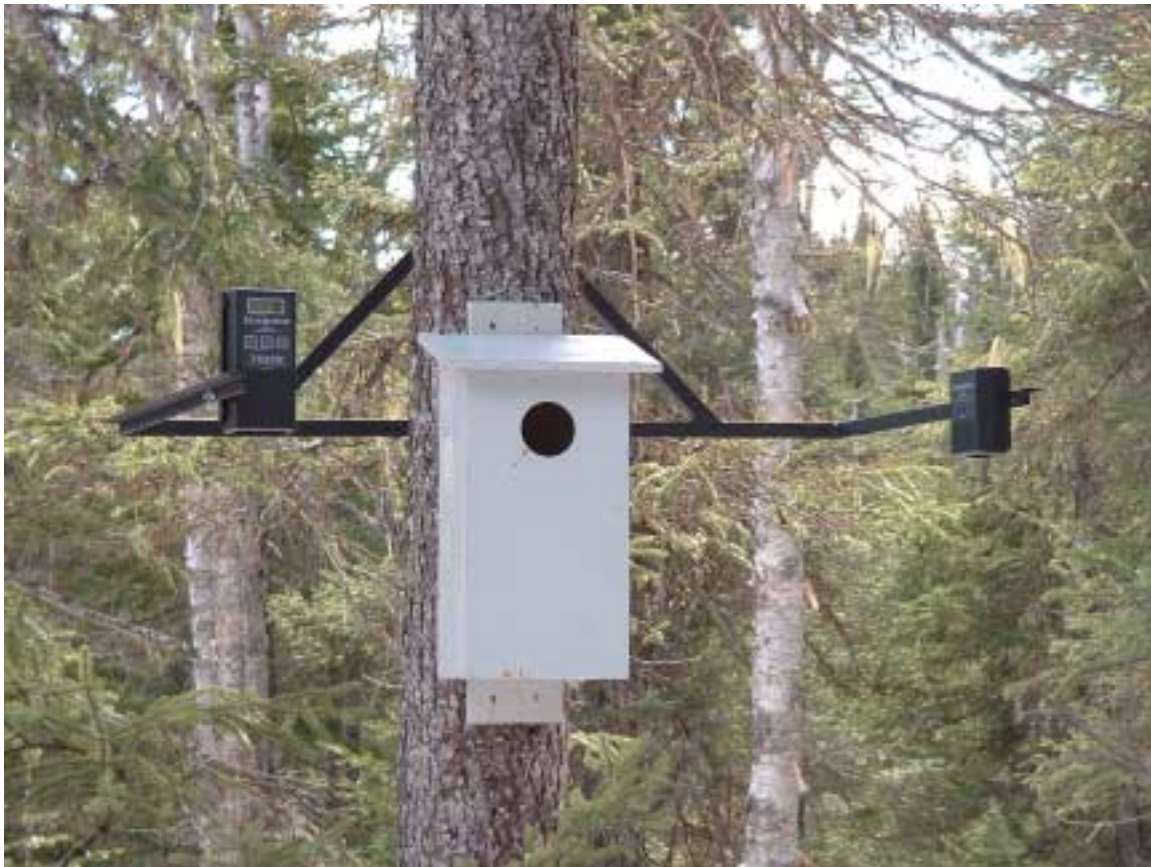
Figure 4: Installation of a Trailmaster TM1550 motion detector for recording the comings and goings from a nesting box of boreal owls.
